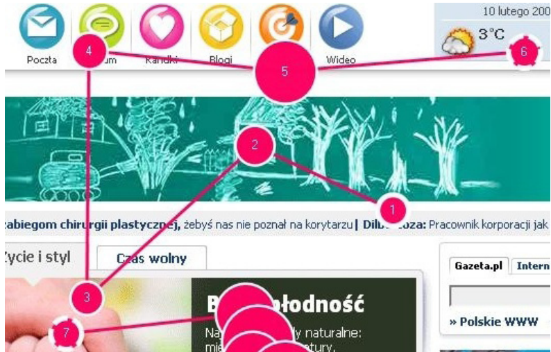
Figure 10. The paths of scanning the website using eyes. The circles depict fixations – the higher the circle diameter the longer the fixation. The lines between circles show the direction of scanning (saccadic eye movement)
